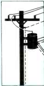
DISTRIBUTION STEP-DOWN TRANSFORMER 0.1 - 1μT, WITH A FAST MAGNETIC FIELD DROP-OFF AT 1/r^3
